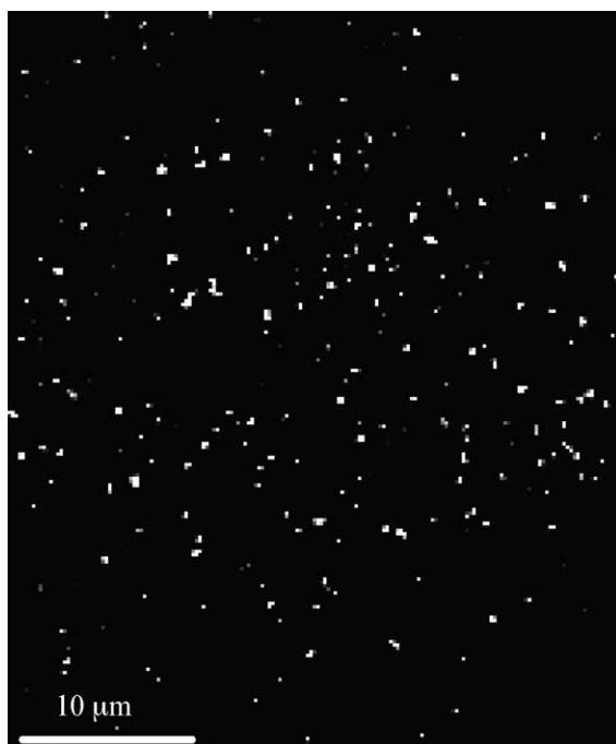
Fig. 2. Native fluorescence images of Npx in pH 7.5 50mM phosphate buffer. Excitation was at 488 nm and 300 W/cm 2 . Exposure time was 20 ms at 2 Hz. Each spot registers a fluorescent molecule.
